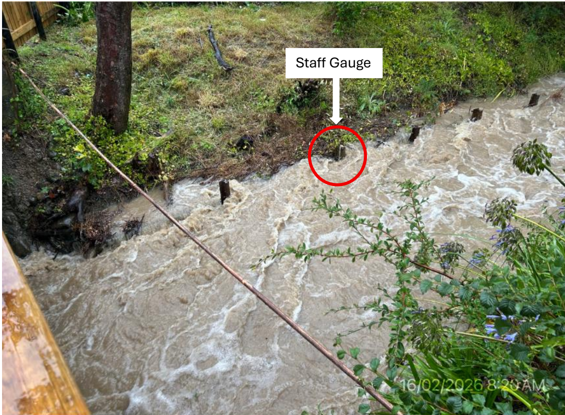
Figure 11 Staff gauge (above and below right), peak flow 1.41m, 8:20am Monday 16 Feb 2026
