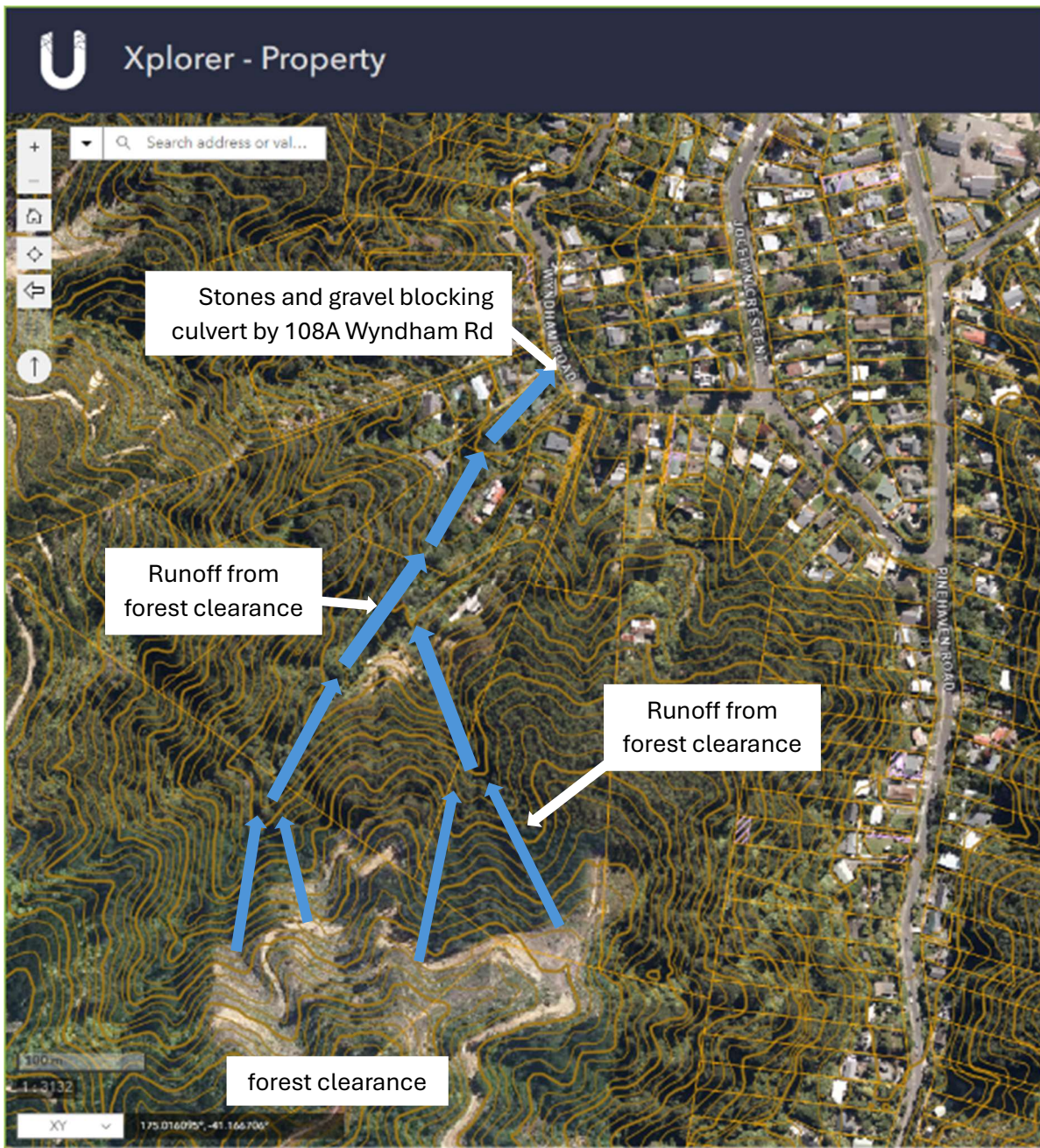
Figure 7 Runoff pathway from recently cleared hillside areas upstream of the blocked culvert near 108A Wyndham Road
