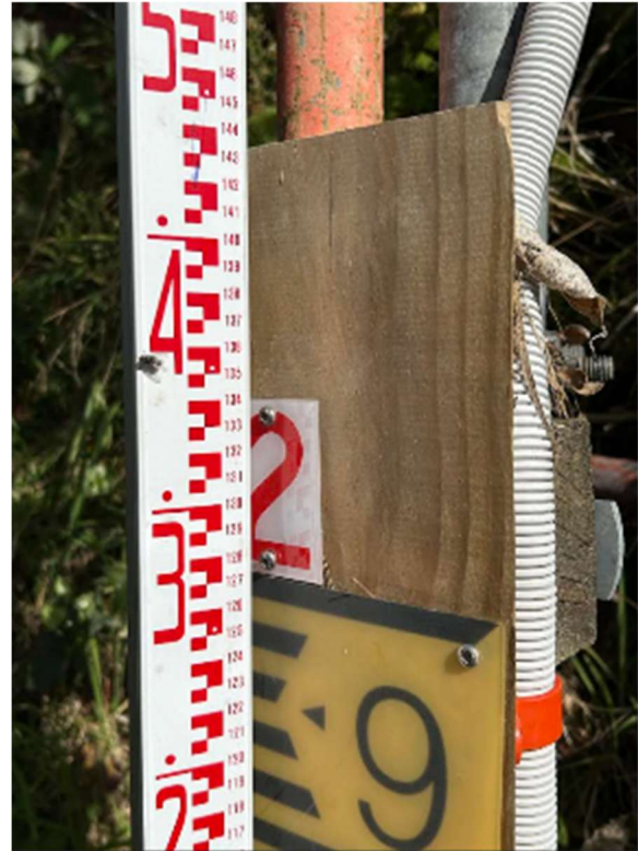
Figure 111 Survey staff shows zero on stream gauge staff is 270mm above bed of the stream
